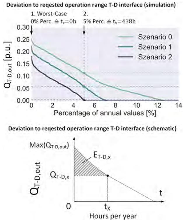
**Fig. 6**  $Q$  deviation to the requested operation range at the T–D interface
